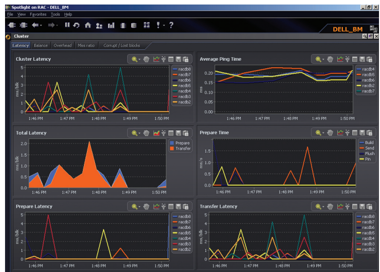
Figure 8. Spotlight on RAC GUI showing cluster-level latency graphs during the eight-node test
