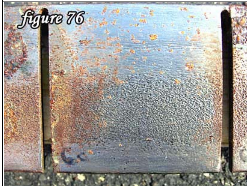
Unfortunately this solvent did not fair too well against the salt on the metal.
