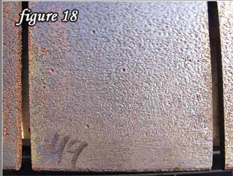
Rep Two Salt Treated (15 Passes of Solvent)
