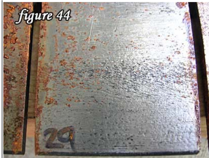
Probably one of the worst test strips seen with very heavy rust formation on the treatment areas.
