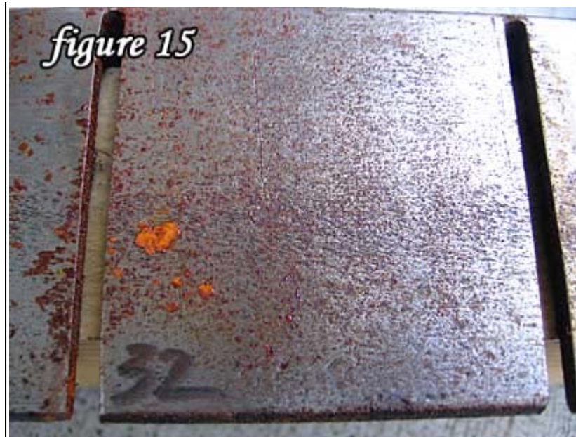
Rep Two No Salt (Control) (15 Passes of Solvent)
