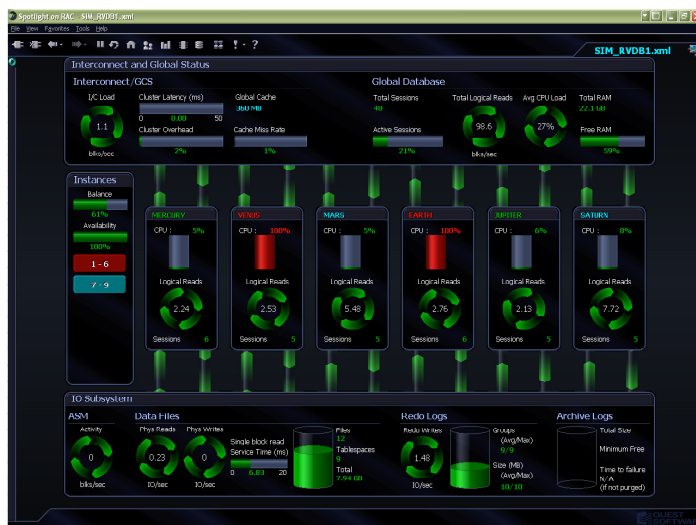
Spotlight on RAC provides a graphical interface for diagnosing performance issues in a RAC environment
