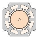
**Cross-Section Perpendicular to Shaft**
