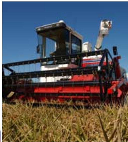
Left • Applying leading technology to rice production: rice harvesting using a Yanmar harvester from Japan, specially imported for RRAPL to harvest small research rice plots
