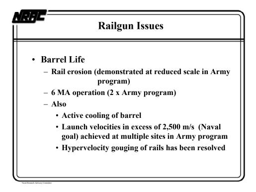
Historically, railgun experiments have been directed more toward exploring the limits of performance than toward issues of durability. Three mechanisms have been identified that can cause rail damage. They are:
