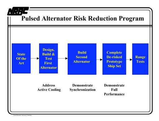
A risk reduction program was laid out to address the issues identified for the pulsed alternator. Once a system design is completed, a full-scale, full featured prototype pulsed alternator should be designed, built and tested to address scaling an particularly active cooling of the rotor windings.
