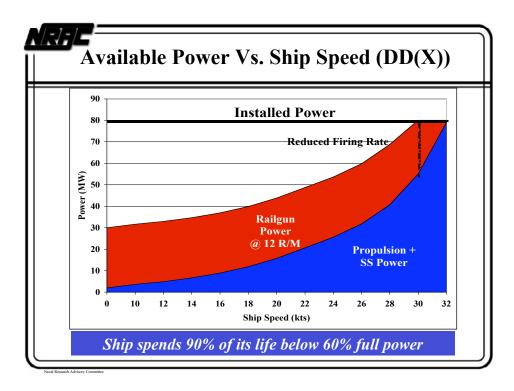
This chart shows very clearly that under all but flank speed conditions there is more than enough electrical power available to operate the gun. We are also convinced that it would be extremely rare – to the point of not happening – that the DD(X) would be providing Naval Surface Fire Support (NSFS) while moving at speeds greater than 25 knots.
