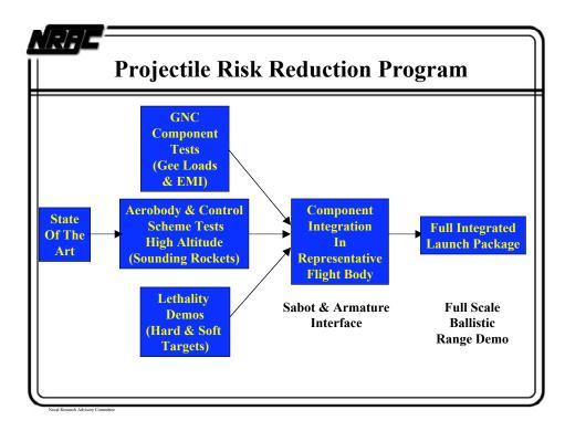
The risk mitigation development schedule has individual low-cost experiments examining the separate component issues. The control and terminal guidance and lethality evaluations can be modeled and then examined in a series of sounding rocket tests at White Sands Missile Range. These will then be brought together in an integration effort before the full-scale ballistic demonstration of the projectile.
