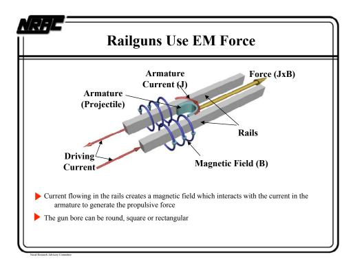
This is a schematic representation of an EM gun. The type shown is a railgun—the most promising technology, as this report will make clear. When a railgun is fired, the current flowing in the rails creates a magnetic field that interacts with the current flowing in the armature—the projectile—to generate propulsive force. A railgun does not burn conventional chemical propellants. The bore of a railgun can be cylindrical, square, or rectangular.
