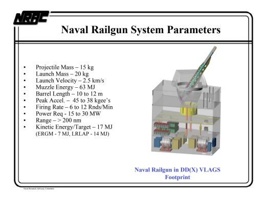
This artist's concept of the Naval railgun system installed in the AGS envelope shows the space available for increased ammunition storage or other needs. The kinetic energy the hypervelocity projectile delivers to the target is compared to that delivered by conventional weapons. In addition to the delivered energy being higher, it would also be more focused and hence more destructive.
