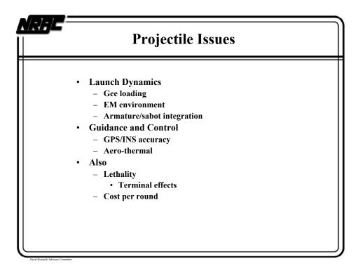
The projectile envisioned for the electromagnetic gun is derived from the HVP development in the Barrage Round Program. That program has already shock tested some guidance, navigation, and control elements to 35 kgee's in addition to actual flight tests at 25kgee's. Also, flechette or preformed fragment dispersal testing was conducted.
