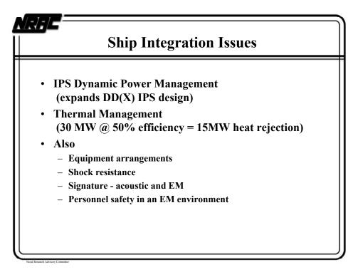
Electromagnetic gun requirements must be considered in the decision and development of IPS. The same consideration applies to handling the 15MW of waste heat that will be generated. The railgun should be located in close proximity to the pulsed alternator to minimize the engineering issues associated with handling 6 MA currents over unduly long cable lengths.
