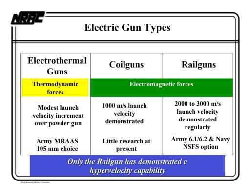
The panel considered three types of electric gun: railguns, coil guns, and electrothermal guns. Electrothermal guns are the most like conventional guns–they use electricity to control the burn rate of the round propelling charge. The principal attribute of this gun is more uniform acceleration of the round. Since the performance is only marginally better than a conventional gun, electrothermal guns cannot satisfy Naval Surface Fire Support (NSFS) range requirements.
