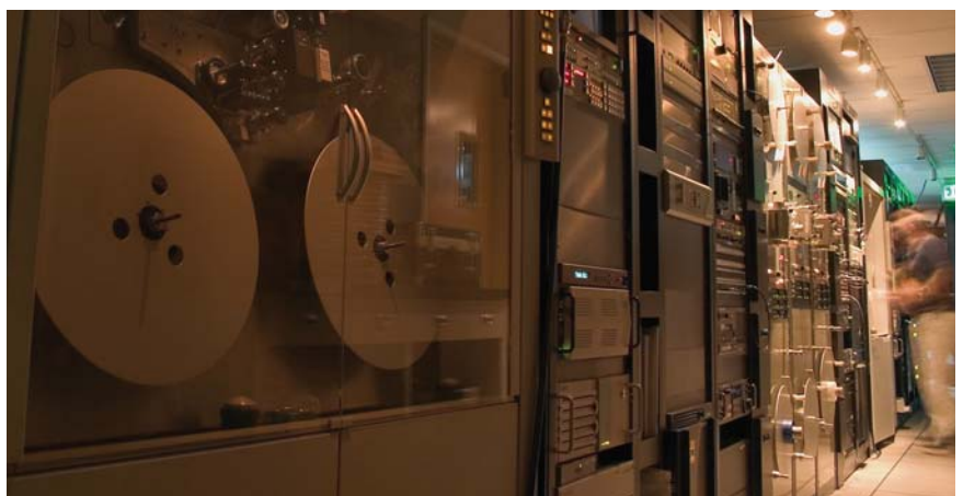
The Spirit Datacine real-time 2K telecine is connected to Foto-Kem's SAN.
