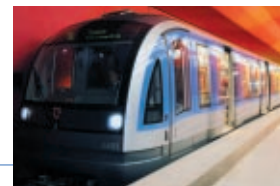
The new underground articulated train is 114 m long and can hold up to 912 passengers.
