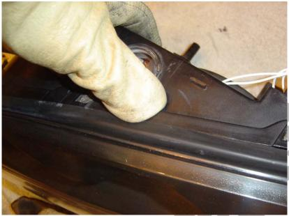
Let the headlight cool and then you can apply the Black RTV High Heat Sealant to the seam all around the headlight. This will help in preventing moisture from getting inside the headlight and causing fogging. Just apply a bead of the sealant as shown below. Be sure to add some sealant to the hole where the wires are coming out the back of the headlight. You want a tight seal.
