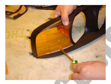
Set aside the black bezel and clear portion of the headlight. Next you will prepare the headlights to take the angel eye rings. You will need to have a drill with a 5/32" drill bit. You will need to drill two holes in the back of the headlight so that the wires from the angel eye rings can exit the headlight. See below on where to drill the two holes:
