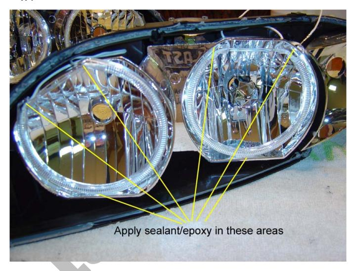
Also, apply a little sealant/epoxy to the wires coming out of the top of the low beam bezel. This will keep the wires from rubbing against the hole. If you are using clear RTV sealant you will want to let that set up for about 12 hours before moving on. You want to make sure it is completely dry.
