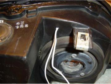
Test fit the angel eyes in the low beam. The ring should fit perfectly inside the low beam bezel. The high beam bezel ring will not fit inside but the bottom will be inside the bezel and the top of the ring will lay on the top of the bezel. See picture below:
