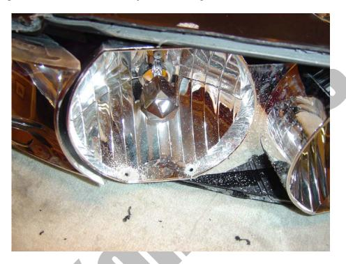
After drilling out the holes clean out the headlight to remove any dust or plastic shavings. You don't want this to be inside the headlight after it is together. I recommend cleaning the chrome bezel with WATER ONLY. Do not put ammonia based products on the chrome. It will take the chrome off. Just use water and a micro-fiber towel to clean the chrome. Clean it good and remove any finger prints or smears.
