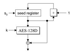
Figure 3-2 – Triple AES Generator (AES-G3)
