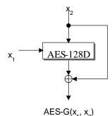
Figure 2-1 – AES-based One-way Function
