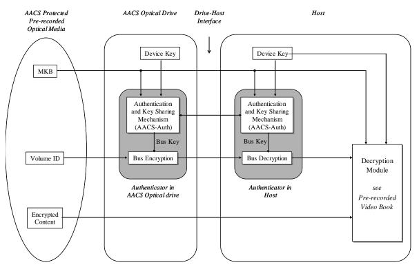
Figure 5-1 – Reading of Volume Identifier in a Drive-Host Configuration
