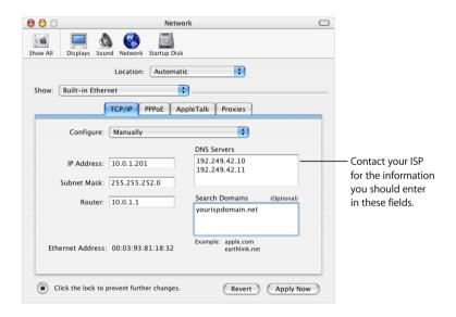
When you configure Ethernet clients manually for a base station that provides NAT over Ethernet, you can use IP addresses in the range 10.0.1.201 to 10.0.1.254.
