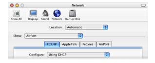
b If you enabled a DHCP server when you set up the base station's network, and the client computer is using Ethernet, choose Built-in Ethernet from the Show pop-up menu and Using DHCP from the Configure pop-up menu in the TCP/IP pane.
