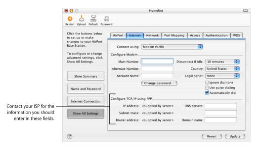
If you have difficulty connecting, you can try to connect at a slower modem speed by choosing Modem (V.34) from the "Connect using" pop-up menu.
