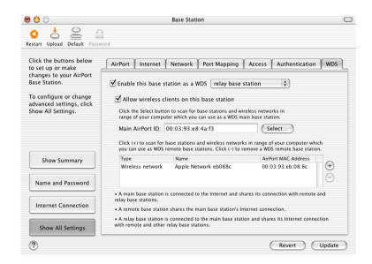
7 Click the Add (+) button to scan for base stations in range of your computer. Click Rescan if the base station you expect to see doesn't appear in the list. Deselect the "Auto configure as a WDS remote base station" checkbox if you want to set up the remote base station manually.
