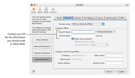
If you are connecting to the Internet through a router using PPPoE and your base station is connected to the router via Ethernet, you do not need to use PPPoE on your base station. Choose Ethernet from the "Connect using" pop-up menu in the Internet pane, and deselect the "Distribute IP addresses" checkbox in the Network pane.
