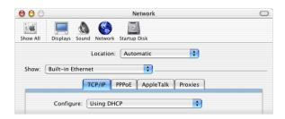
c If you selected "Share a range of IP addresses (using only DHCP)" when you set up the base station's network, you can provide Internet access to Ethernet client computers by setting the client IP addresses manually. Choose Built-in Ethernet from the Show pop-up menu, and choose Manually from the Configure pop-up menu.
