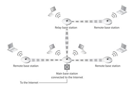
A main base station is connected to the Internet and shares its connection with remote and relay base stations. A remote base station shares the main base station's Internet connection. A relay base station shares the main base station's Internet connection and transfers the connection to other remote or relay base stations.
