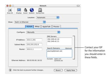
When you configure Ethernet clients manually for a base station that provides NAT services over Ethernet, use IP addresses in the range 10.0.1.201 to 10.0.1.254.
