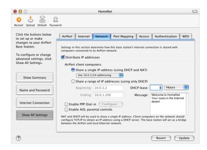
By default, Ethernet client computers share a single IP address using Network Address Translation (NAT). The base station acts as a bridge between the AirPort and local Ethernet networks. When Modem is selected in the "Connect using" pop-up menu in the Internet pane, both the Ethernet LAN (<->>) port and the Ethernet WAN (<->>) port are bridged, and both can share a single IP address using NAT.
