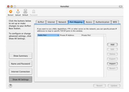
To use port mapping, you must configure TCP/IP manually on the computer that is running the web, AppleShare, or FTP server.
