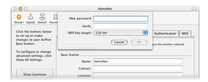
If you choose 128-bit encryption, only computers with 128-bit encryption-capable wireless networking cards will be able to join your network. If you choose 40-bit encryption, computers with 40-bit and 128-bit encryption-capable wireless networking cards will be able to join your wireless network, but they will join with only 40-bit encryption.
