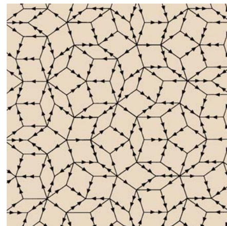
Figure 1 Penrose's planar quasiperiodic tiling. It is formed by a set of two rhombuses with edges of equal length, one with angles of 36° and 144° and one with angles of 72° and 108°. Their edges are marked with single or double arrows, and the rules constrain adjacent tiles to have matching arrow types along their shared
