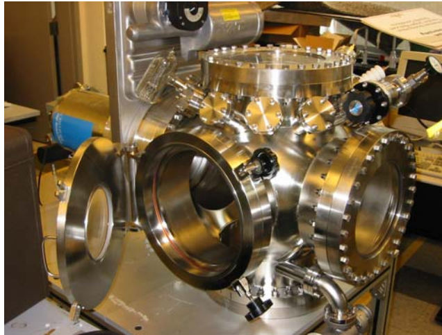
Figure 6. Vacuum system for thruster performance testing.
