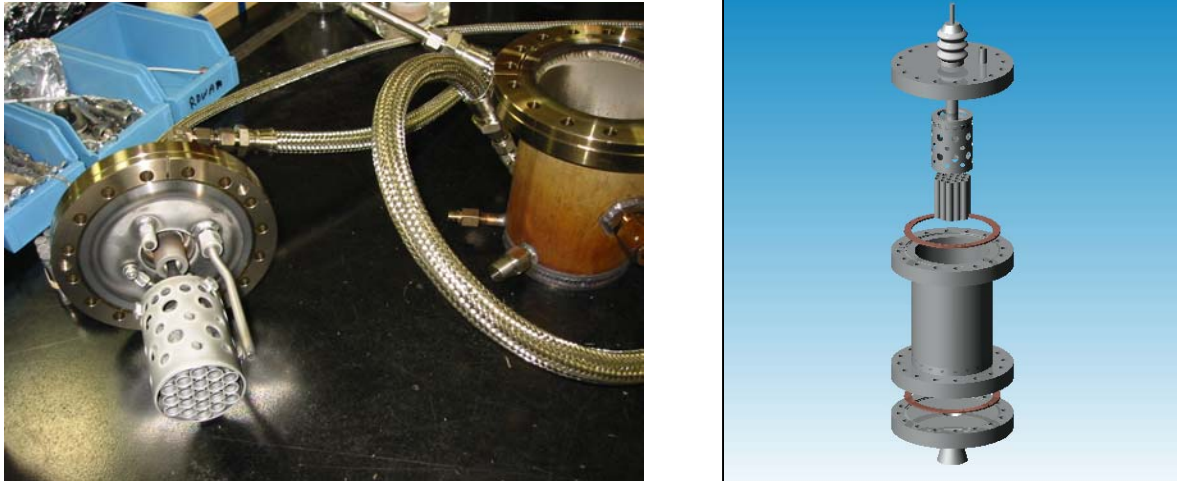
Figure 7. a) Disassembled H 2 /Ne compound hollow cathode gas cell used to generate the BlackLight process (Mills, et al. , 2002) and b) SolidWorks 3D assembly drawing of BLP thruster design.
