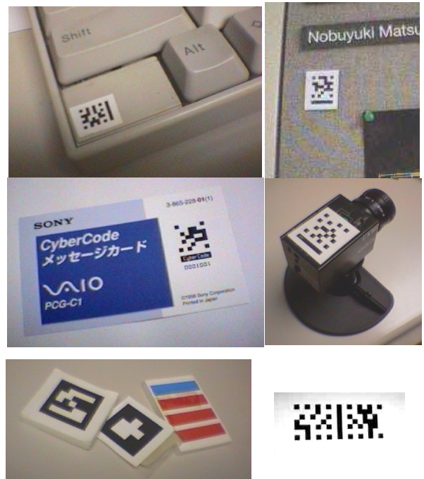
Figure 1: Examples of CyberCode visual tags (top: tags used in several contexts. bottom left: earlier prototypes. bottom right: a concatenated type for more "bits").
