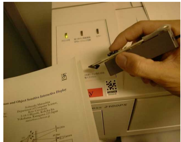
Figure 12: An ID-aware pen is used to perform a “drag-and-drop” between physical objects.
