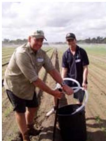
Vegetable growers Mark Anderson and Ben Element measuring the flow rate of knocker sprinklers
