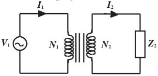
The coils are wound in the same direction, but the current  $I_1$  goes into coil #1 at the same end that  $I_2$  comes out of coil #2, so  $I_2$  gives a flux through coil #1 in the opposite direction to the flux from  $I_1$
