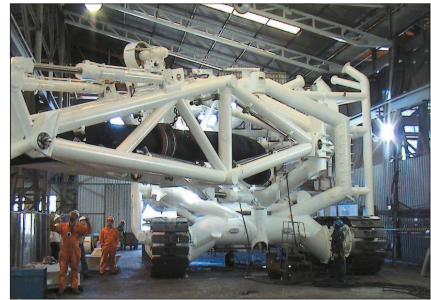
Factory acceptance tests are conducted on the crawler's boom and knuckle prior to installation of the equipment on the diamond recovery vessel, Peace in Africa.
