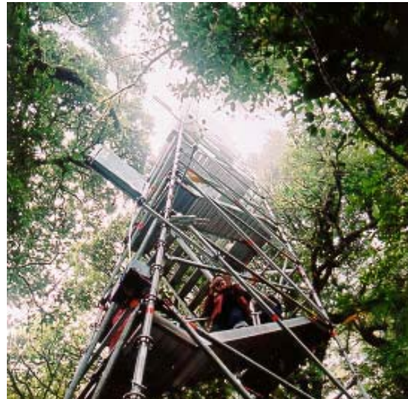
The canopy tower reaches 20 metres into the tree crowns and carries measuring equipment at various heights. Photo: Arnoud Frumau
