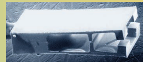
(Left) Laser beam shining out of Keck telescope in Hawaii to produce an artificial guide star. (Above) Microgripper the size of the head of a pin, for use in treating stroke.
