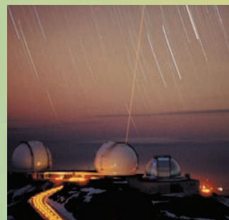
(Left) Laser beam shining out of Keck telescope in Hawaii to produce an artificial guide star. (Above) Microgripper the size of the head of a pin, for use in treating stroke.
