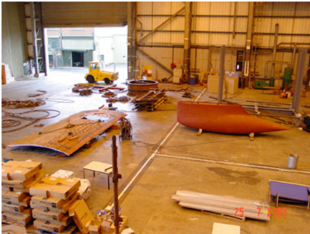
Keel bulb and fin plating
