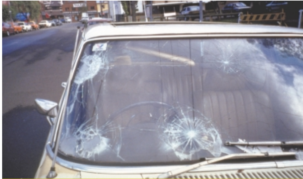
SYDNEY HAILSTORM DAMAGE, APRIL 1999.
