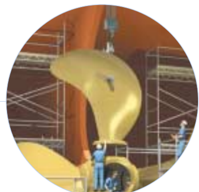
The ABP offers fast and simple installation compared to a monobloc unit.
