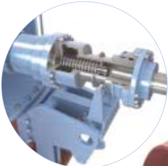
Disconnection of the drive shaft before the thruster is lifted up.
