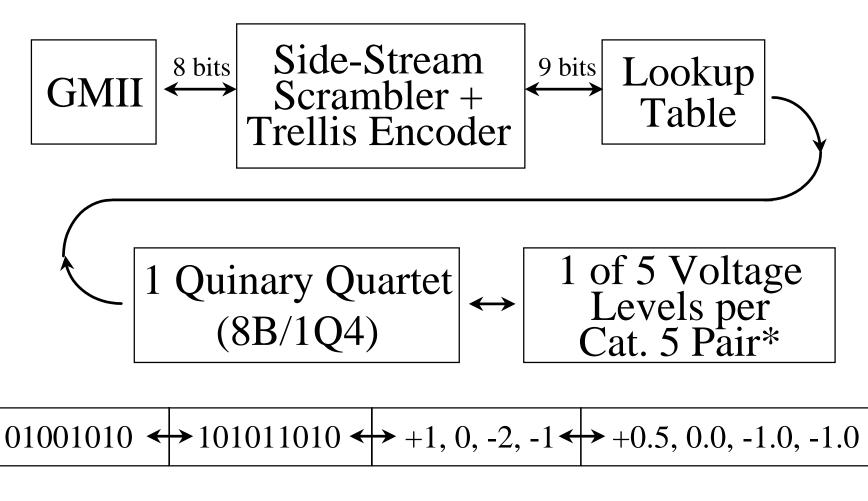
\* Actually 17 voltage levels to reduce emissions by shaping the output
