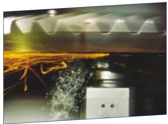
Surface turning a hardened axle drive bevel wheel with PCBN.
