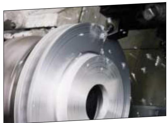
Machining of a MMC brake disc with Syndite PCD.
