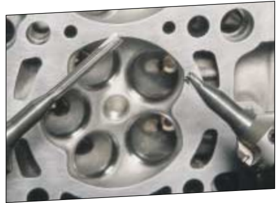
Syndite PCD tipped combination tools for finishing machining.
