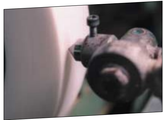
Dressing of a grinding wheel with Monodress.
