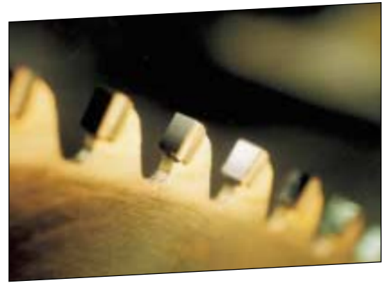
Single-crystal diamond saw teeth used for cutting laminate flooring panels.
