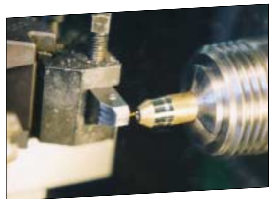
Cutting of an internal thread with a Monodite diamond tool for a component used in dentistry.
