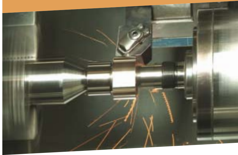
High precision interrupted hard turning with DCN450.
