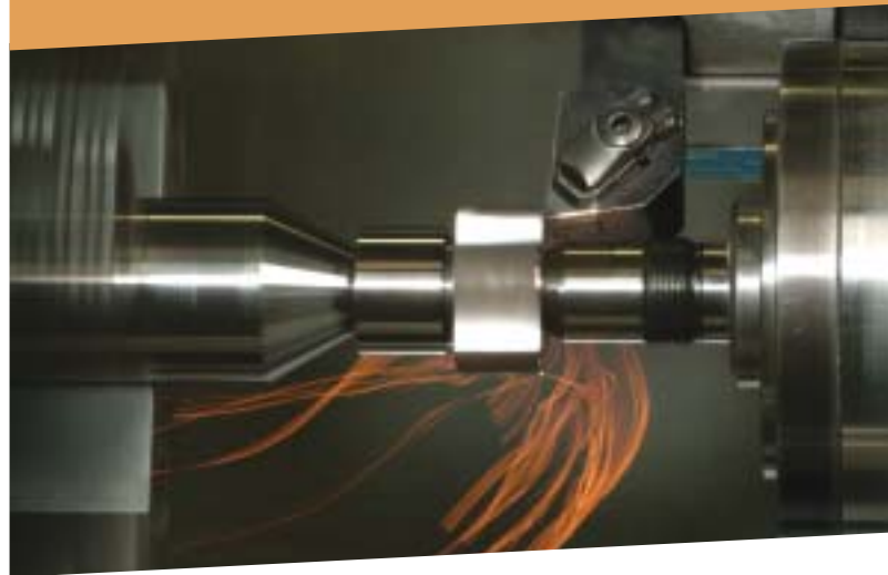
High precision continuous hard turning with DCC500.
