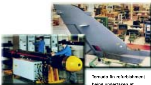
Spearfish torpedo under final assembly. Spearfish is the world's most advanced heavyweight torpedo. It has been developed for delivery to the UK MoD for service in the most modern submarines of the Royal Navy.
