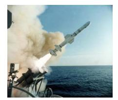
Harpoon Block II provides accurate long-range guidance for land and ship targets by incorporating the low-cost inertial measuring unit from the Boeing Joint Direct Attack Munition (JDAM) program; and the software, mission computer, integrated Global Positioning System/Inertial Navigation System, GPS antenna and receiver from the Standoff Land Attack Missile Expanded Response (SLAM-ER).
