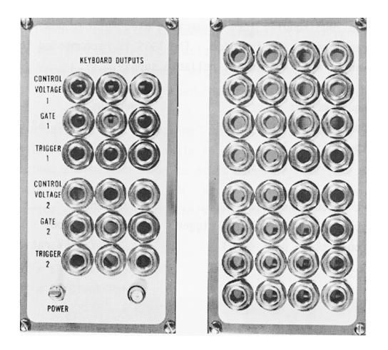
The E $\mu$  2905 Power Supply Modules are complete power systems for E $\mu$  modular synthesizers. The 2905's front panel contains the power switch and pilot lamp, plus multiple outputs for two keyboards. When a keyboard is not connected, the associated system busses can be used for routing any signal by applying via these power supply panel jacks.
