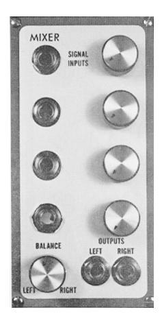
The E $\mu$  2455 Mixer is a four input, stereo output mixer with pan for use within the E $\mu$  modular system. While a mixer is seldom needed in the system as most modules provide input mixing (multiple inputs with attenuators) and output mixing (patching several outputs together in a multiple gives an even mix of the outputs), a dedicated mixer module may prove useful in special situations.
