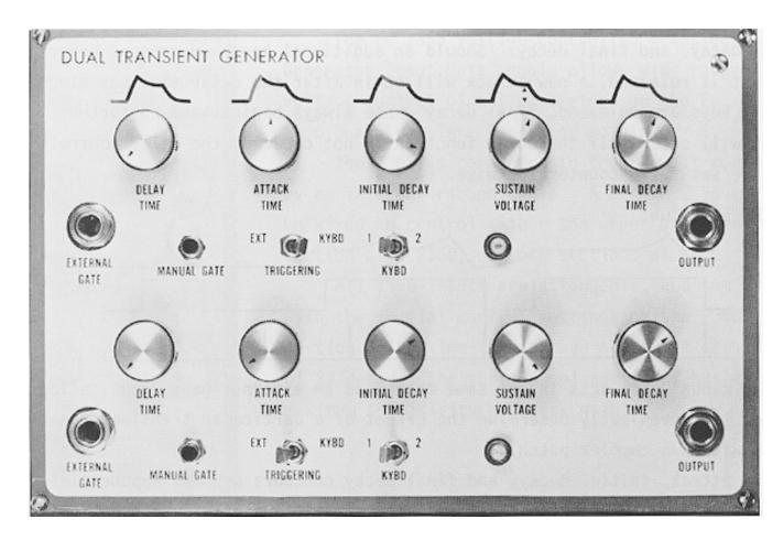
The E $\mu$  2350 Dual Delayed Transient Generator module contains two independent fourphase electronic music transient generators in a single module. It is based on two E $\mu$  1350 submodules.
