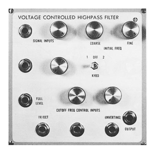
The E $\mu$  2100 Voltage Controlled Highpass Filter is an exponentially controlled highpass filter based on an E $\mu$  1101 submodule.
