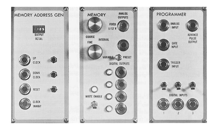
The E $\mu$  2540 Memory Address Generator, 2545 Memory, and 2546 Programmer modules are designed for use together in producing long voltage sequences. The 2540 contains an E $\mu$  1540 submodule, the 2545 contains a 1545 submodule.
