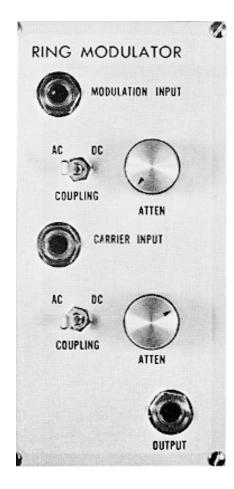
The E $\mu$  2430 Ring Modulator is a balanced modulator for electronic music. It contains an E $\mu$  1430 ring modulator submodule.
