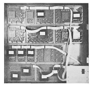
The E $\mu$  Modular Synthesizer System is based around E $\mu$  submodules, compact solid state building blocks providing highly accurate synthesizer functions. The plug-in submodules are designed for maximum flexibility.
