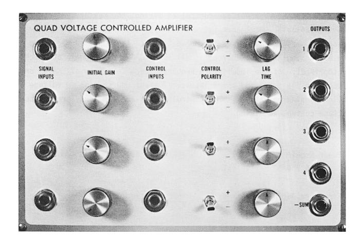
The E $\mu$  2010 Quad VCA module is an array of four independent linear two quadrant multipliers, using two E $\mu$  1010 submodules. It is particularly useful for spatial modulation and voltage controlled mixing.
