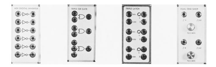
The E $\mu$  2550 Series Logic Modules perform elementary logic functions for use with 2500 series sequencer modules.
