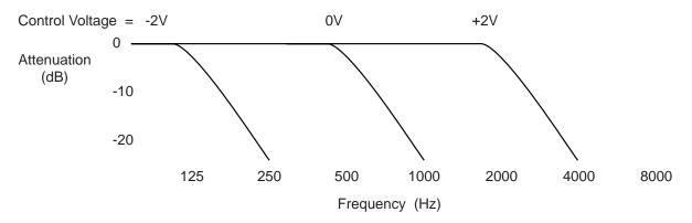
Although maximum accuracy is maintained over the range of 20Hz - 20kHz, the cutoff frequency may be brought as low as 1Hz for special effects.
