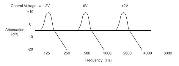
As the Q approaches maximum setting, the filter breaks into oscillation, producing a pure sine wave. Lowest distortion occurs with the Q control set barely into the oscillation region.
