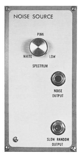
The E $\mu$  2400 Noise Source produces random audio and control signals for use in electronic music. It contains an E $\mu$  1400 noise source submodule.
