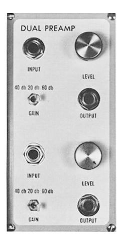
The E $\mu$  2420 Dual Preamp is a dual variable gain preamplifier for use in interfacing external signals to the modular synthesizer system. It is not intended to replace studio preamps for other purposes. The two amplifiers are completely independent.
