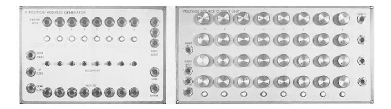
The E $\mu$  2510 and 2520 modules perform the basic potentiometer matrix functions of early sequencers. The 2510 is an eight position (3 bit) up/down presetable, cascadable counter; the 2520 is a 4 by 8 potentiometer matrix.
