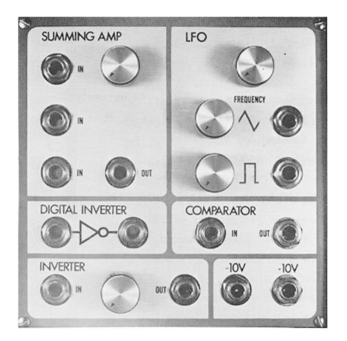
The E $\mu$  2451 Potpourri Module is a multipurpose module designed to add a variety of useful functions to small or medium sized modular systems.
