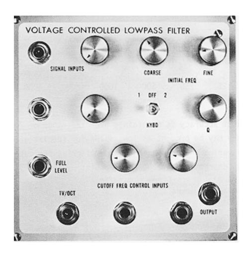
The E $\mu$  2100 Voltage Controlled Lowpass Filter is an exponentially controlled lowpass filter with variable Q for electronic music applications. It contains an E $\mu$  1100 VCF submodule.
