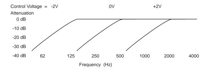
Although maximum accuracy is maintained over the range of 20Hz - 20KHz, the cutoff frequency may be brought lower for special effects.
