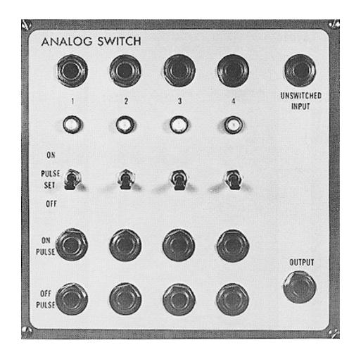
The E $\mu$  2530 Analog Switch is a four channel digitally controlled summing buffer with an additional uncontrolled input for cascading switch sections. The output is the algebraic sum of the voltages appearing at the inputs to activated channels plus the voltage at the unswitched input. Signals at the off inputs are rejected at better than 80 dB. Whenever an input channel is "on", the corresponding lamp is lit.
