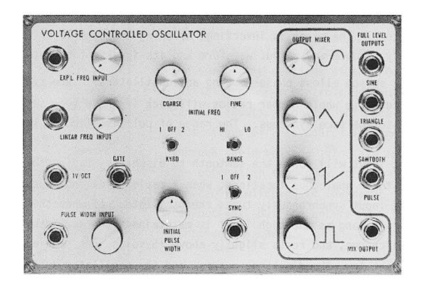
The E $\mu$  2200 Voltage Controlled Oscillator is a complete, four waveform, exponentially and linearly controlled oscillator with an output mixer. It is exceptionally stable and accurate for use with full size synthesizer keyboards. It contains an E $\mu$  1201 VCO submodule, and an E $\mu$  1210 wave converter submodule.
