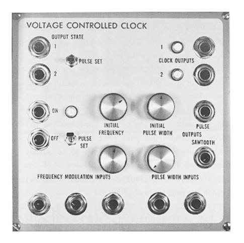
The E $\mu$  2500 Voltage Controlled Clock module is a low frequency sawtooth/ pulse VCO with special gating capabilities, based on the E $\mu$  1500 submodule.
