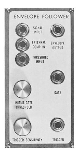
The E $\mu$  2440 Envelope Follower module is a conventional envelope detection circuit with slope and level comparators to derive trigger and gate signals. It contains an E $\mu$  1440 submodule.
