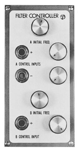
The E $\mu$  2145 Filter Controller allows voltage control of the frequency of two banks of E $\mu$  2140 Resonant Filters. Each bank of filters may contain from one to four 2140 units connected in any series or parallel combination. The bank center frequency will be determined by the 2145 controller while the formant shape will remain unchanged.
