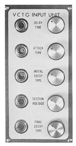
The E $\mu$  2355 Voltage Controlled Transient Generator Input Unit module allows wide range voltage control of all parameters on the E $\mu$  2350 Dual Transient Generator module.
