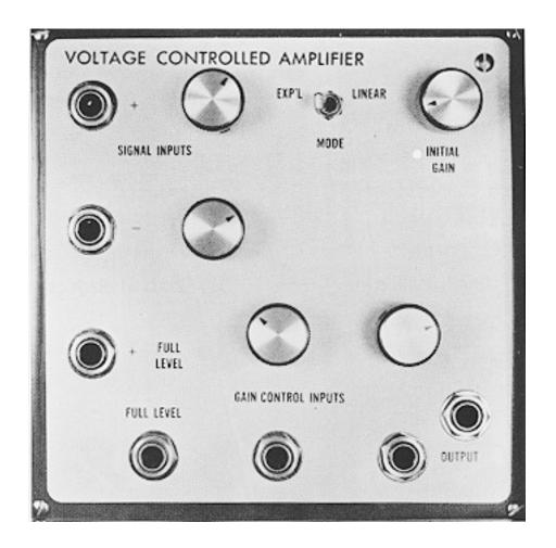
The E $\mu$  2000 Voltage Controlled Amplifier is an exponentially and/or linearly controlled amplifier for envelope shaping or control functions. It contains an E $\mu$  1001 VCA submodule.
