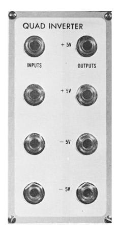
The E $\mu$  2450 Quad Inverter is an array of four independent analog signal inverters. The output of the inverter is the inverse about 0 volts of the input signal. Thus a voltage V at the input gives -V out, and sine waves are put 180° out of phase.
