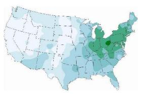
**Isoline** (also called **isopleth**) **maps** use lines to connect points of equal value, such as temperature, rainfall, or elevation. Lines of equal temperature are called **isotherms**, lines of equal rainfall are called **isohyets**, and lines of equal elevation are called **contours**. Contour lines are often used on topographic maps.
