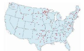
**Dot-density** (also called **dot**) **maps** place individual points on a map to correspond with occurrences of a particular feature or data. Clusters of dots show where the features or data are concentrated.
