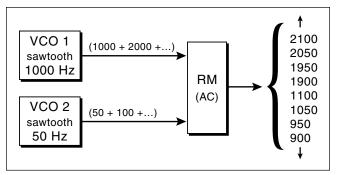
This is why the ring modulated output has a characteristic gong-like sound. A gong has non-harmonic resonances at different places along its surface, giving a similar effect.
