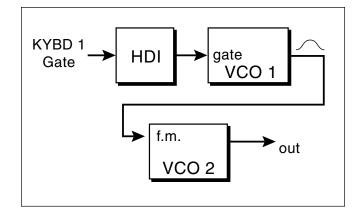
VCO 1, the gated VCO, is normally off, since the hex digital inverter (q.v.) outputs a digital "one" to its gate input. When any key is depressed, the output of the HDI goes to a digital zero, and VCO 1 synchronously begins a slow sine wave output at the sine jack. This is used to modulate the frequency of VCO 2, giving a precisely reproducible trill at VCO 2's output. If the key is just tapped, exactly one cycle of the trill will occur, then VCO 2 will return to its original frequency.
