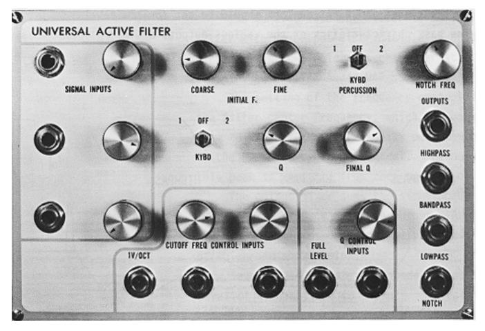
The 2120 Universal Active Filter is a multimode resonating filter with simultaneous highpass, bandpass, lowpass, and notch outputs (all at the same  $f_c$ ). It has three attenuable signal inputs, two attenuable  $f_c$ control inputs and one at 1V/octave, one attenuable Q control input and one at 1V/ factor of two, and several features which will be discussed in a moment.
