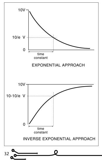
Clearly, then, a decay is still significantly short of its approach value well after the time constant elapses. For example, a final decay with a time constant of 10 seconds will give a total glide time of about 30 seconds. (The time constant is precisely definable, however, while the "total glide time" depends on the sensitivity of your ear). The attack phase, being cut off at 10/12 of its approach value, lasts about 1.7 time constants.
