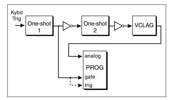
The following diagram shows the synchronization among the different signals in the patch:
