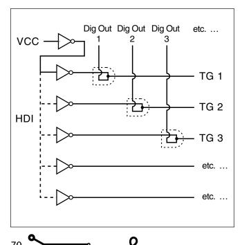
Sometimes, of course, you may want the option of programming a particular digital output high in several consecutive addresses for the purpose of sustaining a note or rolling over notes without attacks. To have both types of gating available, we generally use digital output 2, "and"-ed with the clock, to gate one TG, and digital output 3 to gate a second TG directly. Thus, staccato, legato, and sustains are all possible, depending on how you program the two gating bits.
