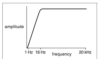
This is obtained from the "noise output" jack when the "spectrum" pot is full left. The attenuation of the theoretically flat spectrum at low frequencies is due to the necessity of filtering out any DC component in the output. Listen to white noise through a VCF with the Q set just short of oscillation. As you sweep f<sub>c</sub>, you will hear the VCF output whistle smoothly through the entire audio spectrum, indicating the presence of every frequency in the noise.
