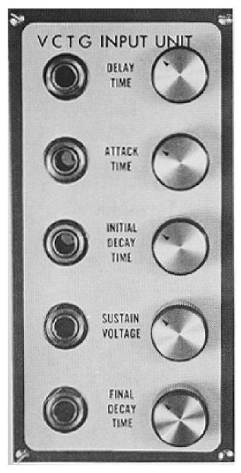
The 2355 Voltage Controlled Transient Generator Input module makes it possible to control all five of the TG parameters with input voltages; the VCDTG submodule is always voltage controlled, but it receives its control voltages only from the pots on the module when the VCTGI is not used. The VCTGI simply adds attenuated control voltages to the voltages obtained from the appropriate pots.
