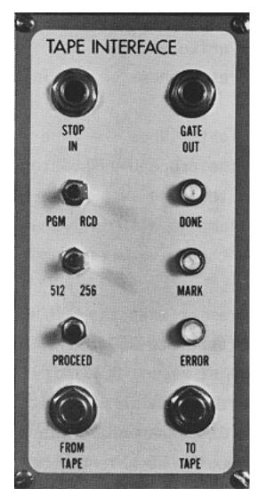
The 2547 Tape Interface makes it possible to store the contents of memories as audio signals on recording tape, and to reprogram the memories from the tape recorder at any time. With this module, you can accumulate a library of sequences in permanent, nonvolatile form.
