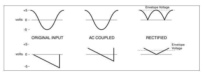
negative portions of the waveform are reflected through zero volts, thus becoming positive. After rectification, the resulting DC offset (the envelope) is extracted by a simple four-pole lowpass filter (f<sub>c</sub> about 25 Hz) Notice that these three functions (AC coupling, rectification, and lowpass filtering) could be performed in a patch with a VCHPF, a ring modulator, and a VCLPF. The EF simply performs these functions (and others, as well) in one module. See the diagram above.
