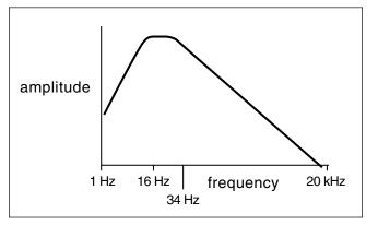
Notice that the low filtered noise is no lower in volume than the white noise, even though it has been filtered. The circuitry boosts the low filtered output to accomplish this, the
