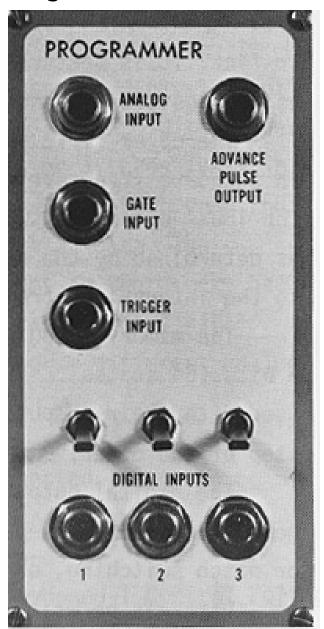
The 2546 Programmer has three inputs which are used in the programming of control voltages from a keyboard. These are the
