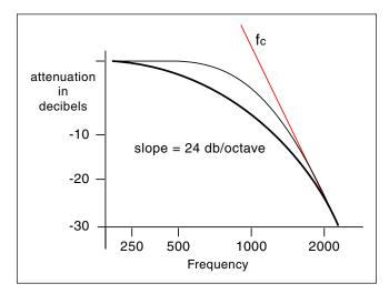
First off, what is this good for? For one thing, filtering of razzy tones will give mellower, more spectrally pure tones, and this can be done to any extent desired. Run a sawtooth wave through a VCF with the Q off (full left), and notice the effect of the initial  $f_c$  pots. As  $f_c$  is lowered (counter-clockwise), the timbre of the output gets less razzy, approaching and finally reaching the pure sine wave timbre.
