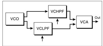
Here, the only frequencies which cannot reach the VCA are those which can't pass either the LPF or the HPF—the result is a band-reject filter. In this case, the LPF  $f_c$  is lower than the HPF  $f_c$ . If vice-versa, all frequencies are passed and some are boosted (this could be called a 'band-boost' filter; not really a filter at all, and we haven't looked into it much (maybe it's just the thing for your application).
