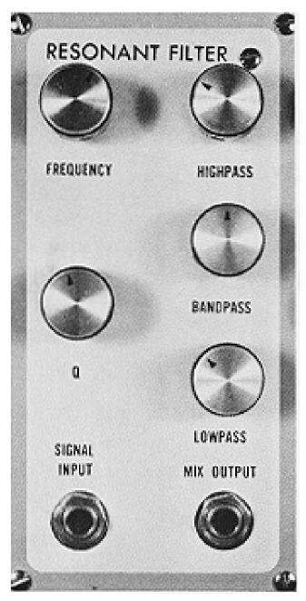
The 2140 Resonant Filter is one module which is capable of producing the same two-pole mixed-function filter characteristics as the UAF/QVCA pair just discussed, but lacking the voltage-controllability features.
