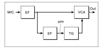
It is possible with this patch to remove sharp attacks or long decays from the microphone signal by setting the parameters on the TG appropriately. If an electric guitar is used instead of a microphone through the DP still), the plucked attacks can be removed from the guitar envelope, giving a radically different voice to the guitar.
