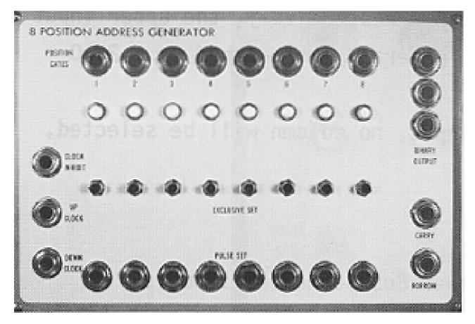
The Eight-Position Address Generator and the Voltage Source Output Unit together comprise the type of sequencer commonly used in most synthesizers— the potentiometer matrix. However, because of the separation of the two modules, and certain special features, the 8AG/ VSOU pair is somewhat more versatile than other pot matrix sequencers.
