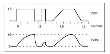
The response to a gate, as shown in this diagram, is useful as a voltage controlled exponential attack/release transient generator. (With the shape pot in between the two extremes, the response to a sudden change in input voltage is a linear ramp initially, which becomes exponentially rounded, starting partway through the slide).
