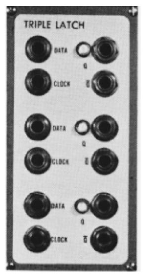
The 2552 Triple Latch contains three identical digital latches. A latch is essentially a digital sample & hold; when the "clock" input changes from digital zero to digital one, the digital value currently applied to the "data" input is sampled and held, or "latched", at the Q output; and its digital inverse (its "complement"), is latched at the  $\overline{Q}$  output (pronounced "Q-bar'). These outputs remain indefinitely at the digital values most recently latched.
