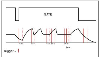
Study carefully the conditions under which new attacks are initiated. Notice that a delayed trigger has no effect if it occurs during an attack phase (or without a high gate). Also, many triggers in quick succession may have
