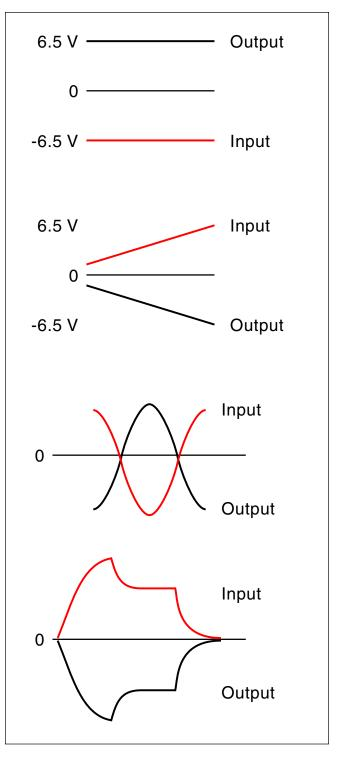
The input jacks are pre-patched (via their shunts through precision resistors) to the +15V and -15V power supplies. The supply connections and resistor values are such that the upper two input jacks receive -5V through their shunts, and the lower two inputs receive +5V. Thus, +5V is available from either of the upper two outputs, and -5V from either of the lower two outputs when no patch cord is in
