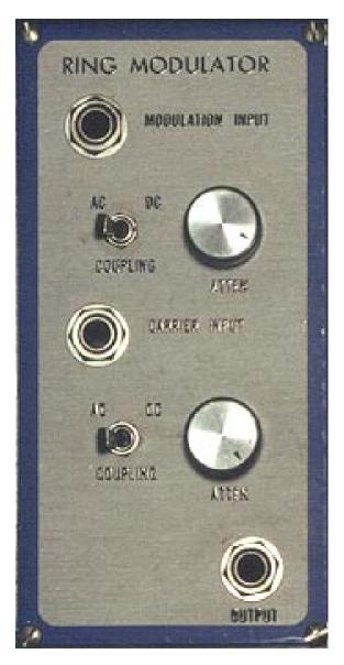
The ring modulator is typically used as a source of enharmonic spectra—complex spectra whose components are not harmonically interrelated. The name comes not from the sounds it makes, but from the diode ring used in early circuits. The output of the ring modulator is the algebraic product of the two inputs. The product of two sine waves is the sum of two new sine waves, with frequencies equal to the sum and difference of the original frequencies:
