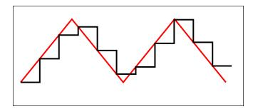
This gives a stepwise ascending and descending glissando at VCO 3's output. If VCO's 1 and 2 are sync'd, the glissando will be repetitive.
