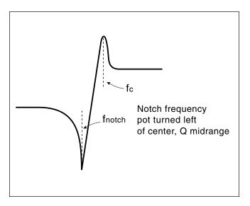
As this formation is swept up and down in frequency space, the effect is quite strange, being sort of a combination of "wah-wah" (Q) and "phase-shifter" (notch).
