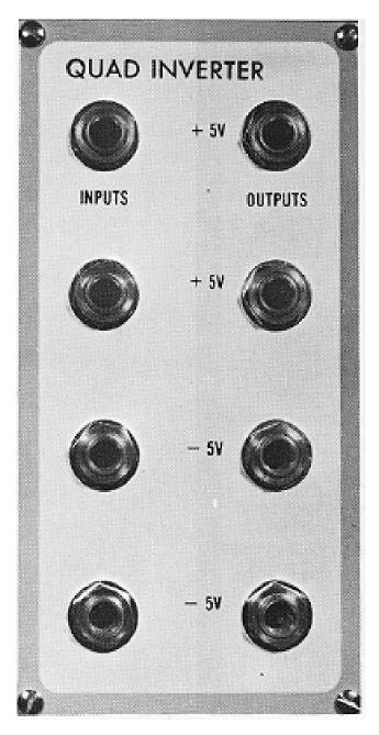
The 2450 Quad Inverter contains four independent analog inverters. When a voltage V is applied at an input, -V appears on the corresponding output jack. Since the inverters respond at any frequency from zero Hz to super-audio, they will invert any audio or subaudio input. These drawings show a few possibilities:
