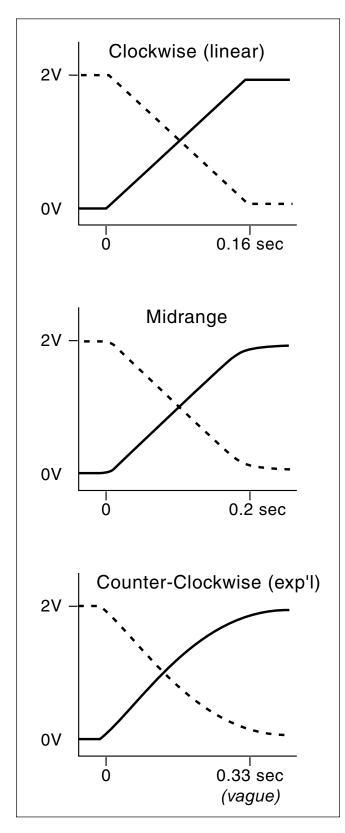
The rate pot controls the overall rate of the approach. In linear mode, the slew rate is adjustable from 1V/10 msec (counter-clock-wise) to 1V/sec (clockwise). Notice that the overall glide time is longer for the same rate setting in exponential mode than in linear mode.
