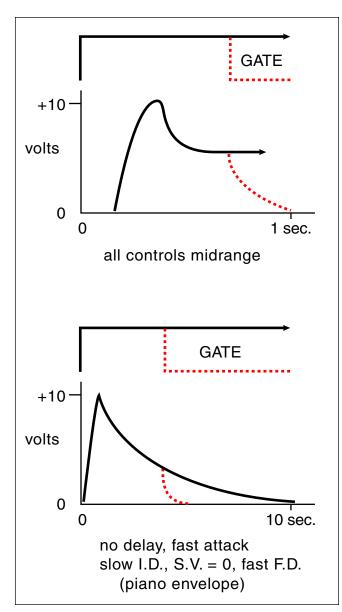
When a monophonic keyboard (q.v.) is used, additional triggers are often produced without the gate ever going low; specifically, this happens either when a lower key is depressed without releasing an upper key, or when two keys are depressed and the lower is then released. It is necessary that a transient be able to respond (with the appropriate delay) to such additional triggers.
