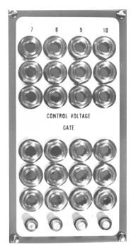
The 4050 Keyboard is a modular digital keyboard with true polyphonic capability up to ten voices. The physical keyboard is identical in outward appearance to the 4000 Monophonic Keyboard; however, in the 4050 series, several modularized functions are available as options, corresponding roughly to separate circuit boards interconnected within the 4050 keyboard cabinet.
