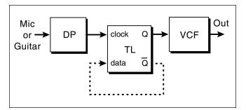
The output signal will be one octave lower in pitch than the input signal, provided the gain of the DP is high enough to give excursions greater than 2.5V in its output. If either Q or  $\overline{Q}$ is patched into the "clock" of the second latch, its Q and  $\overline{Q}$  outputs are then two octaves below the original signal. This division can be performed indefinitely with more latches.
