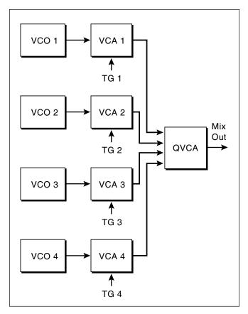
If the four VCO's are tuned to track together, say, at intervals corresponding to the fundamental and the next three harmonics of a note, the envelope of each harmonic can be independently controlled by its own TG. If all the TG's are triggered from the keyboard, the delay time allows any of the envelopes to have the same shape but to be displaced in time, the only limitation being that the final decays will all begin simultaneously when the gate falls.
