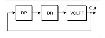
The output of this patch can be a very bizarre sound whose pitch and timbre are drastically affected by the  $f_c$  of the filter and the "% reverb" setting on the DR. If you like the feedback effect, try voltage-controlling it. Remember that you can obtain voltage controlled reverb percentage simply by mixing the 100% reverb output with the original signal in a QVCA.
