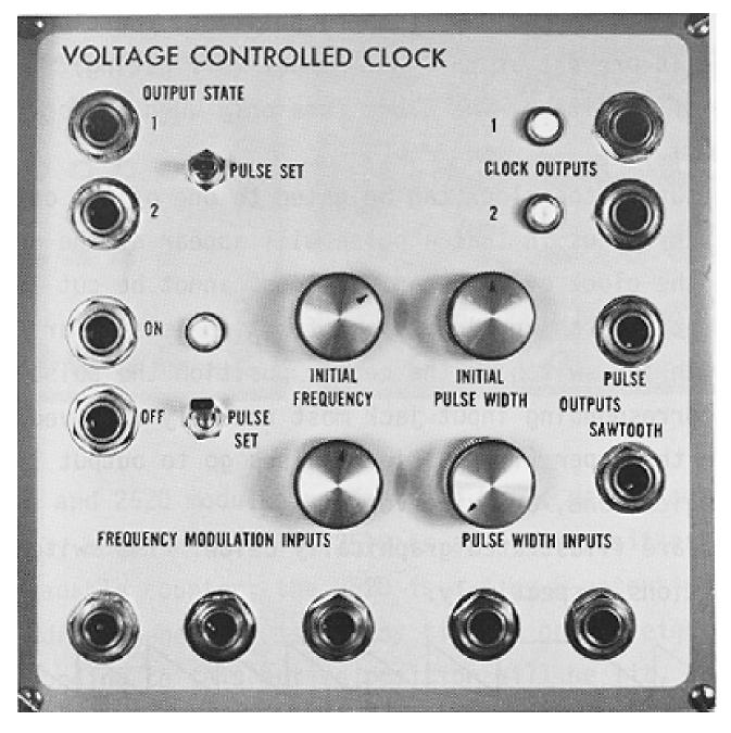
The 2500 Voltage Controlled Clock is a sawtooth/pulse VCO designed primarily for low frequency (0.001 Hz to 500 Hz) clocking of sequences. It contains a 1500 Voltage Controlled Clock submodule with the following unique features: a digital pulse output, synchronous on/off gating, and synchronous routing to either of two output channels. The module also outputs routed pulse and sawtooth waveforms. The frequency
