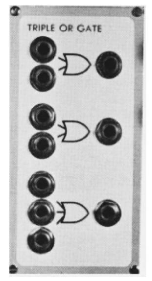
The 2551 Triple Or Gate (accent on the or) contains three independent "or"-gates; two have two inputs, and the third has three. The output of each ."or"-gate is a digital one if any of the inputs is a digital one, and zero only if all the inputs are zero. Specific applications will be discussed as they arise—in general, the TO is used whenever a digital event is to occur in response to one of several other digital events.
