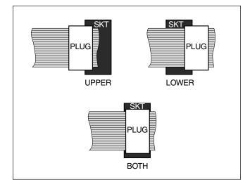
The DIP plug on the DTG itself is plugged into its socket in the normal way. One VCTGI can control any number of TG's; here is a wiring scheme which gives VCTGI 1 control over the upper TG's in three DTG'S, and gives VCTGI 2 control over the lower TG's;
