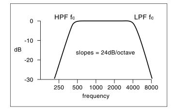
Apply a control voltage simultaneously to a control input of the LPF and to a noninverting control input of the HPF, and adjust the attenuators to about the same control level. The band-accept filter will now respond to a change in this control voltage by chang-
