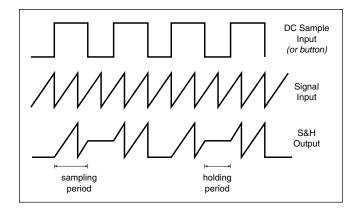
(When the 'manual sample' pushbutton is depressed, its effect is the same as a high level an the DC sample input).
