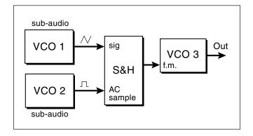
If the triangle is much lower in frequency than the pulse wave, a step function results at the S&H output:
