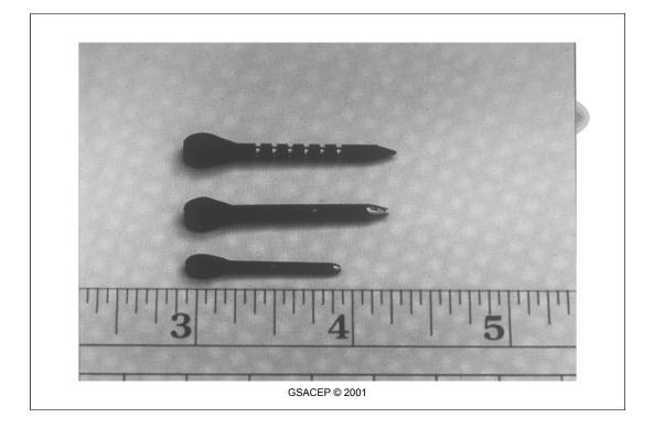
These flechettes were designed to be used with either chemical or biologic agent, (either wet or dry) which would fill the grooves or drill-holes.
