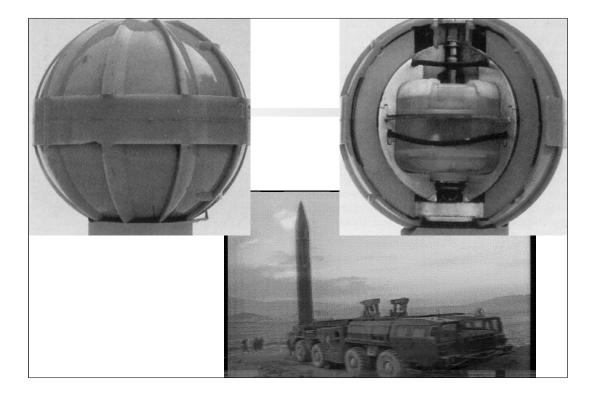
Biologic agents can also be disseminated using aerosols contained in bomblets that can be released from missiles, such as this SCUD-D, which can carry 2-3000 bomblets.
