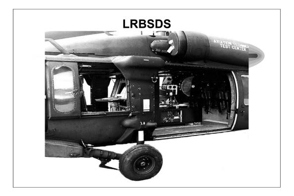
The Long Range Biological Standoff Detection System (LRBSDS) uses <u>laser-induced fluorescence</u> to detect aerosol clouds w/ particles of the right size range, up to 30 km away - the improved version will be able to reach out to 100km. It can differentiate smoke, pollen, and pollution from BW aerosols.
