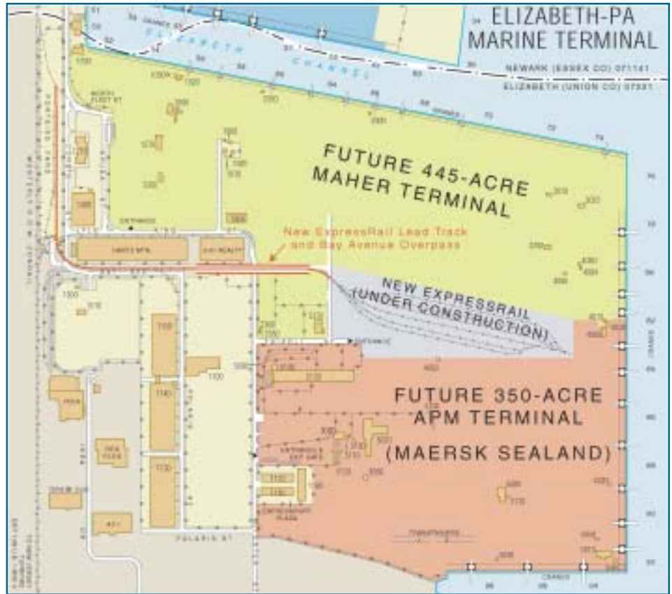
ExpressRail (Elizabeth-PA Marine Terminal): A new 70-acre ExpressRail intermodal terminal is under construction at the Elizabeth-PA Marine Terminal (above). The new on-dock rail facility will have direct access from both the consolidated Maher Terminal and the expanded APM Terminal. The first phase of the new ExpressRail will open in 2004. When fully completed in 2005, the terminal will have a capacity of up to 1 million container lifts per year.
