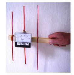
Suggested starting dimensions: Reflector: 370 mm long, 65 mm behind the radiator. Director: 290 mm long, 75 mm in front of the radiator.
