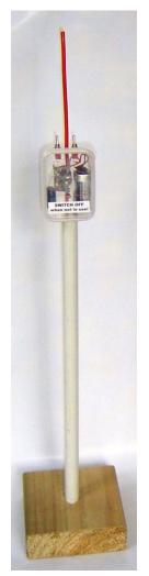
The Transmitter Unit on its stand (using plastic pipe)
