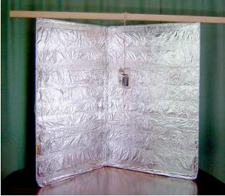
Two pieces of hardboard about 700mm by 500mm are held together by a hinge made of wide sticky plastic tape. The two pieces of hardboard must be kept about 2mm or 3mm apart when applying the tape to allow for easy folding. The tape is applied to both sides of the hardboard. The "fold" is along the 700mm dimension. One whole face of the two boards including the fold is then covered with aluminium foil, glued on.
