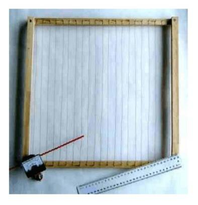
When the glue has set, small nails are tacked at 20 or 30 mm intervals along two opposite sides of the frame as shown in the photograph.
