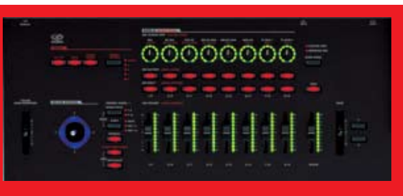
FIG. 2: The Mixer & Modulation section is packed with assignable knobs, sliders, and buttons for controlling synth parameters, audio and MIDI tracks, and even external hardware and software.
