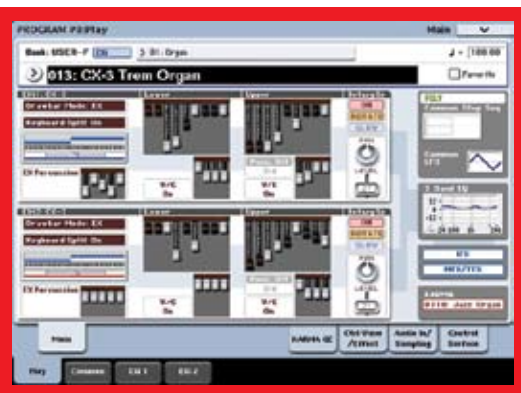
FIG. 4: CX-3 effectively duplicates every control parameter of a Hammond organ and a Leslie cabinet, from drawbar and split settings to independent horn and rotor speed.
