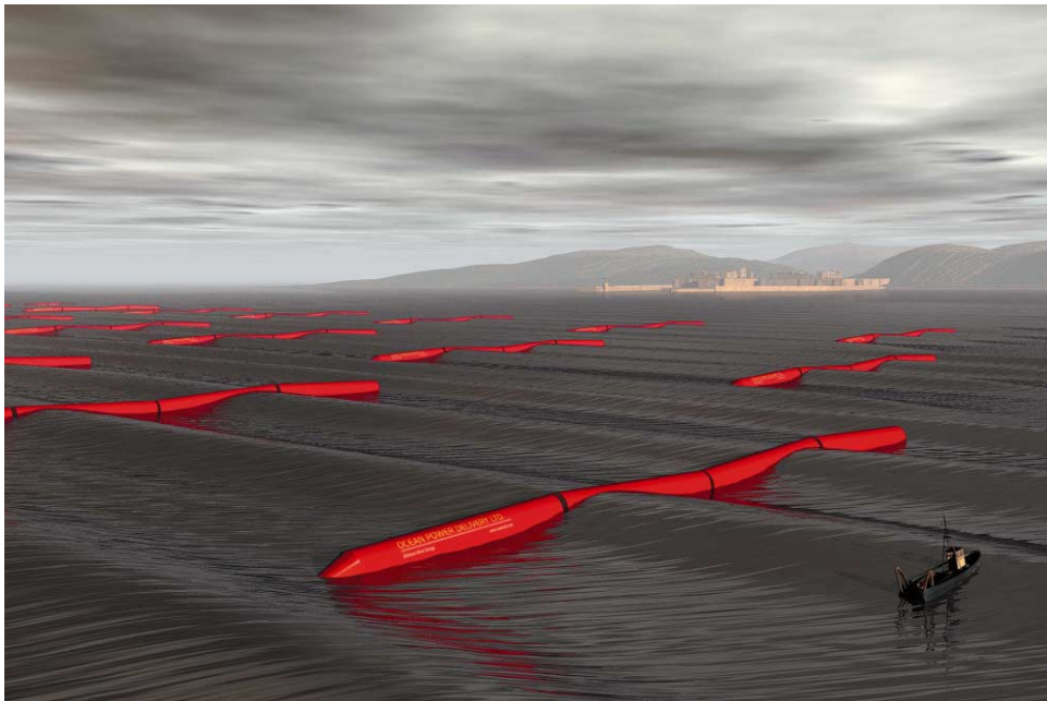
FIGURE 15.6 Artist's impression of the Pelamis Wave Energy Converter (Source: Ocean Power Delivery).
