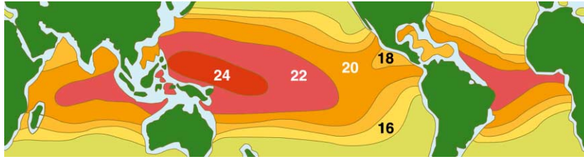
FIGURE 16.1 The area available for OTEC and the temperature difference. (Source: Xenexys Inc).
