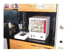
Bacterial Incubator at UMass Dartmouth. The device is capable of incubating bacteria in gel medium or broth due to its oscillating shelves.
