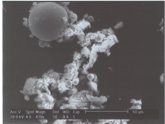
Figure 2. An SEM image from sample 2 shows a number of spherules along with other dust particles.
