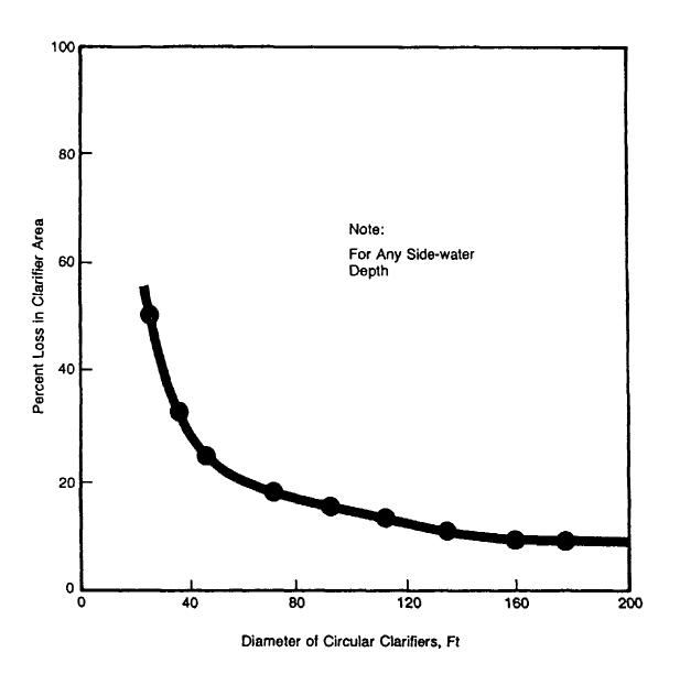
Figure 11-2. Effective surface area adjustments for inlet—outlet losses in circular clarifiers.
