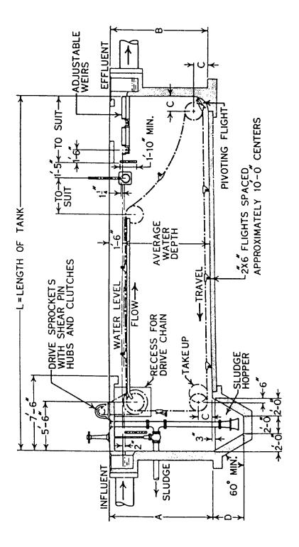
Figure 11–3. Typical rectangular primary sedimentation tank.
