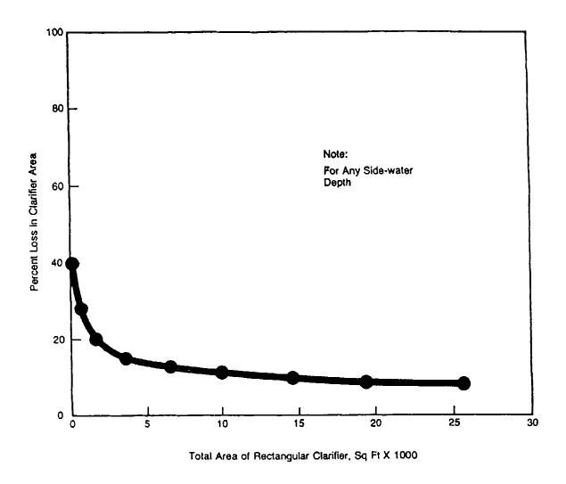
Figure 11-1. Effective Surface area adjustments for inlet—outlet losses in rectangular clarifiers, L:W=4.
