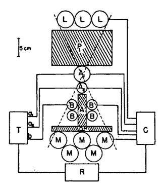
Figure 1: Experimental arrangement used in the determination of the disintegration curve of mesotrons.
