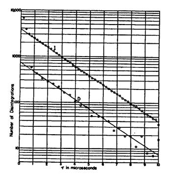
Figure 3: Differential (D) and integral (I) disintegration curves of mesotrons obtained from the combined data of the lead, brass, and aluminum absorbers. The straight line through the experimental points for the differential curve is drawn according to the method of least squares.
