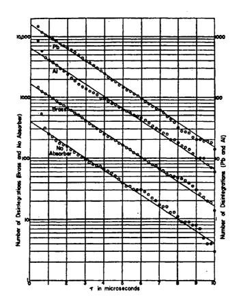
Figure 2: Integral disintegration curves of mesotrons obtained with lead, aluminum, brass, and no absorber in A.
