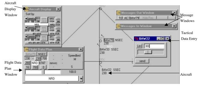
Figure 11 - The Prototype Air Traffic Control Simulator
