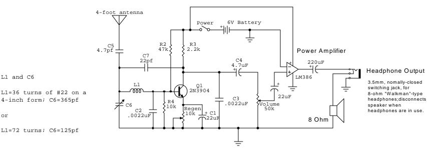
Procedure: Tune R1 until oscillation occurs; back off until is ceases. Now tune C6 for a station, retuning R1 as necessary.
