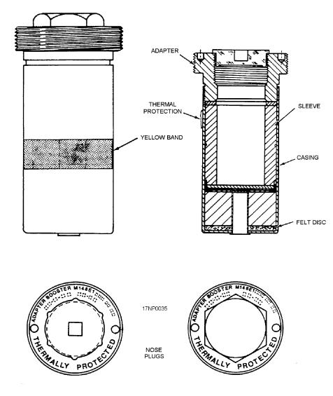
Figure 1-4.—Adapter-booster M148/E1 (series).
