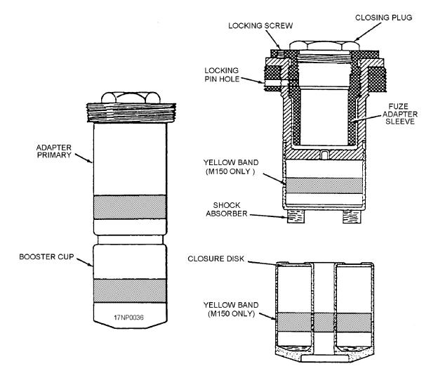
Figure 1-5.—Adapter-booster M150/T46 (series).
