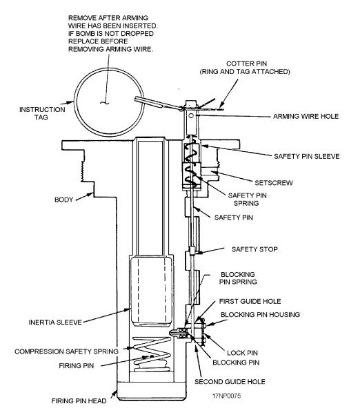
Figure 1-37.—Mk 89 Mod 0 bomb spotting charge adapter.
