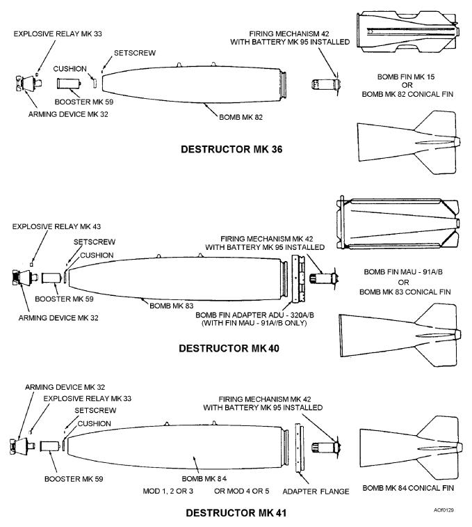
Figure 1-29.—Typical destructor configurations.
