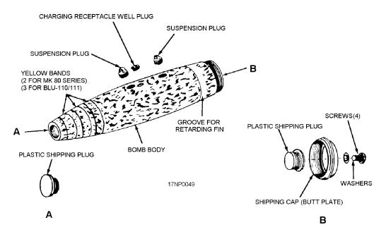
Figure 1-15.—LDGP bomb Mk 80 (series)—exploded view (shipping configuration).
