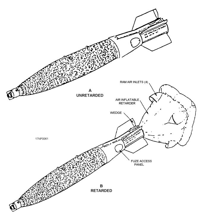
Figure 1-24.—Typical BSU-85/B air-inflatable retardable fin with high and low drag configurations.
