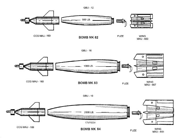
Figure 1-27.—Typical guided bomb unit configurations.
