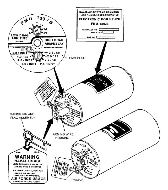
Figure 1-8.—FMU-139 (series) electronic bomb fuze.
