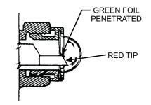
B. MK 339 MOD 1 FUZE SAFE/ARM INDICATOR PIN IN ARMED POSITION
