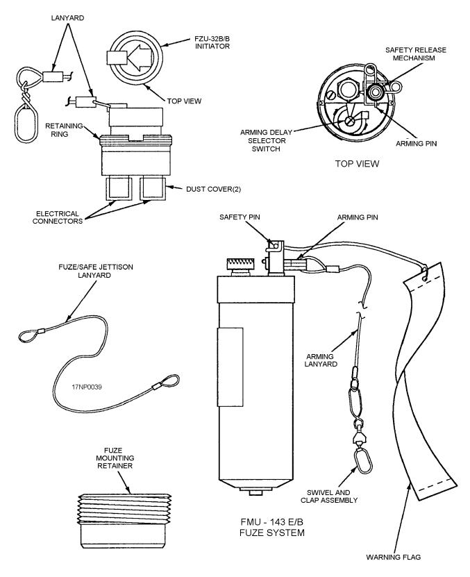
Figure 1-7.—FMU-143E/B electric tail fuze.
