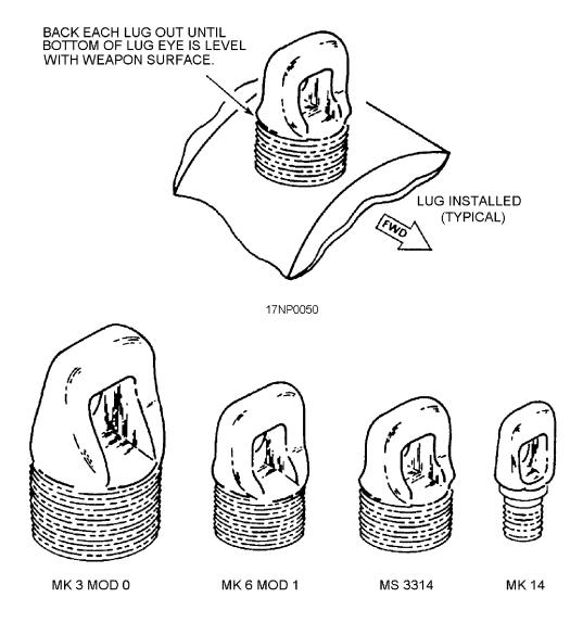
Figure 1-16.—Suspension lug installation.
