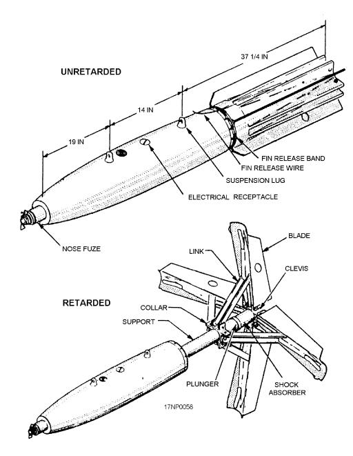
Figure 1-21.—Mk 15 fin with Mk 82 bomb body.
