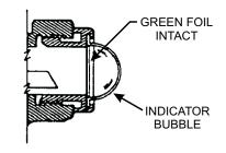
A. MK 339 MOD 1 FUZE SAFE/ARM INDICATOR PIN IN SAFE POSITION A7. The M904 arms and functions by <u>rotation of</u> <u>arming vanes and alignment of internal</u> <u>components</u>.
