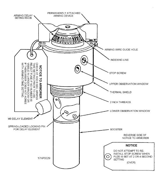
Figure 1-1.—Mechanical impact nose fuze M904 (series).
