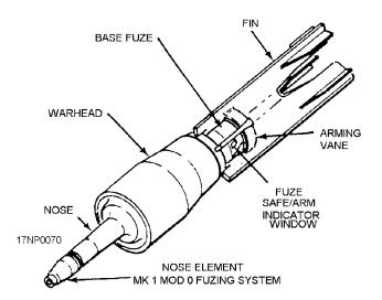
Figure 1-32.—Antitank bomblets Mk 118 Mod 0 and Mod 1.
