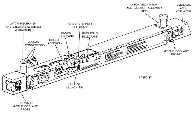
Figure 3-26.—LAU-93/A guided missile launcher.
