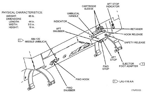
Figure 3-22.—LAU-116/A guided missile launcher.
