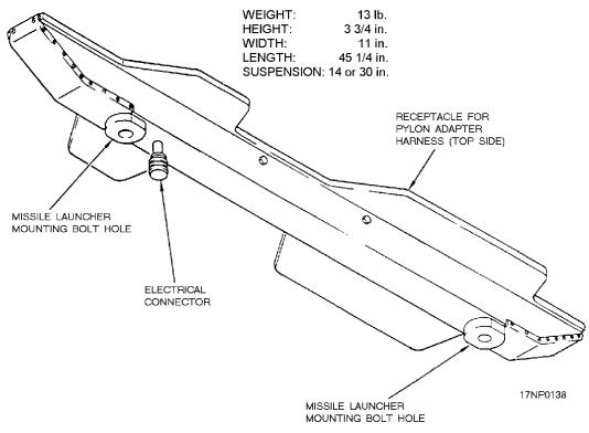
Figure 3-27.—ADU-299/E missile launcher adapter.
