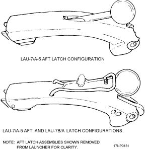
Figure 3-20.—Aft fairing latch assembly.
