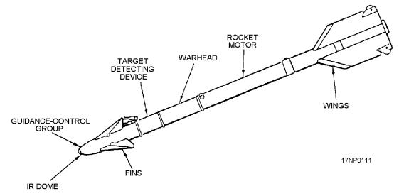
Figure 3-1.—Typical air-to-air guided missile.
