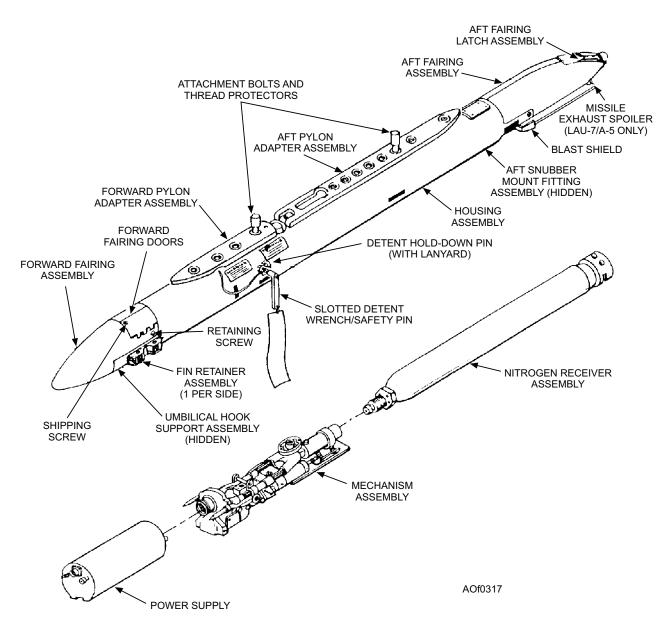
Figure 3-17.—LAU-7/A (series) guided missile launcher.
