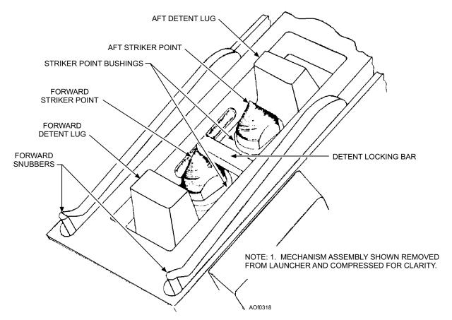
Figure 3-18.—Mechanism assembly detent and snubbers.
