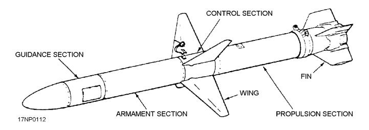
Figure 3-2.—Typical air-to-surface guided missile.
