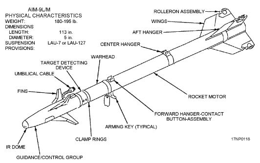
Figure 3-8.—AIM-9 series Sidewinder guided missile.
