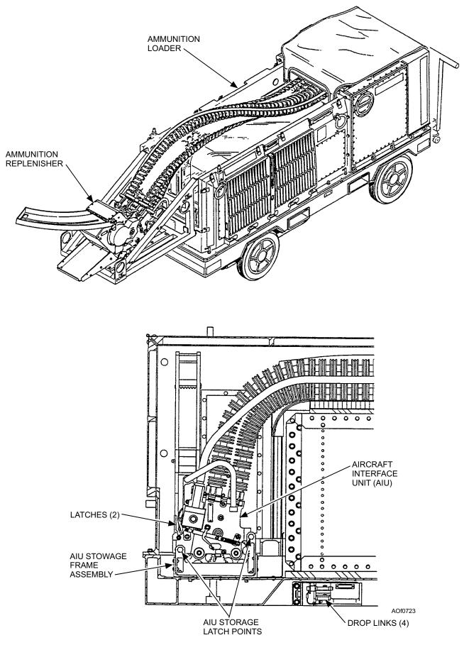
Figure 7-23.—AIU Stowage Frame Assembly Position.
