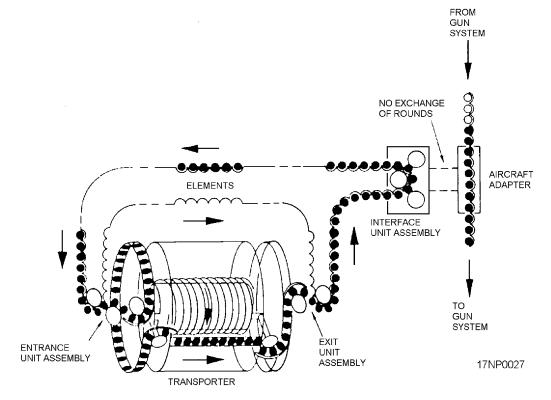
Figure 7-18.—Ammunition flow in bypass mode.
