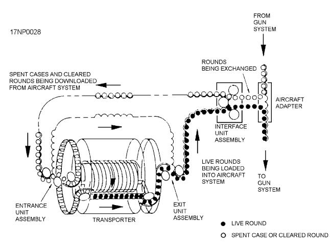
Figure 7-19.—Ammunition flow in load/download mode.
