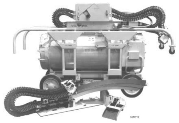
Figure 7-12.—Linkless ammunition loading system (LALS).
