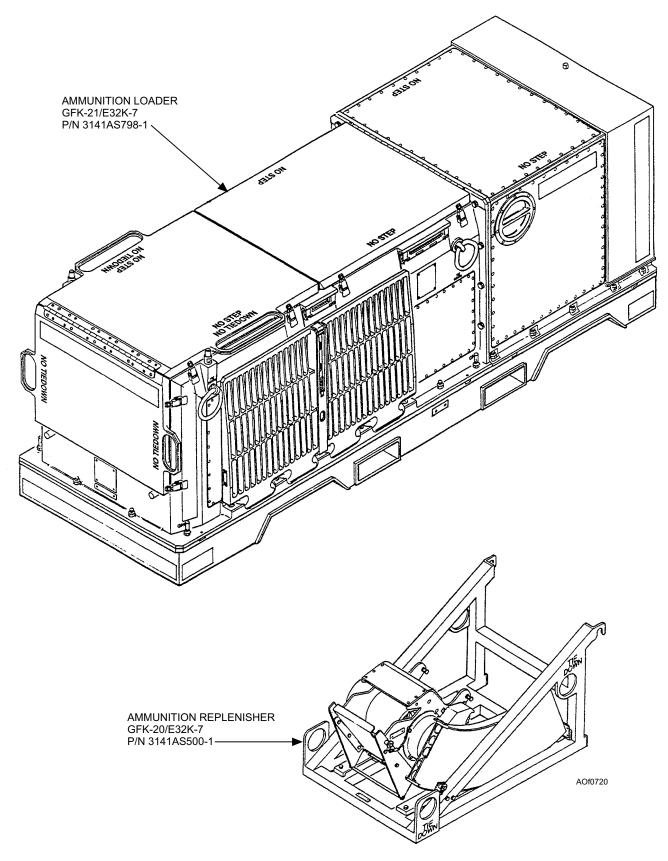
Figure 7-20.—Linkless Ammunition Loading System (A/E32K-7).
