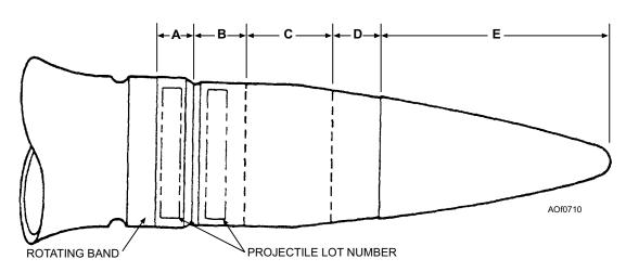
Figure 7-10.—Color Coding and Marking for PGU Configuration Ammunition.
