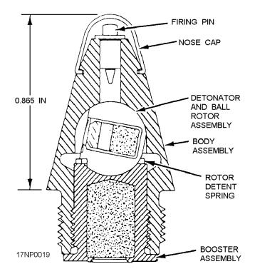
Figure 7-3.—M505A3 point-detonating fuze (unarmed).
