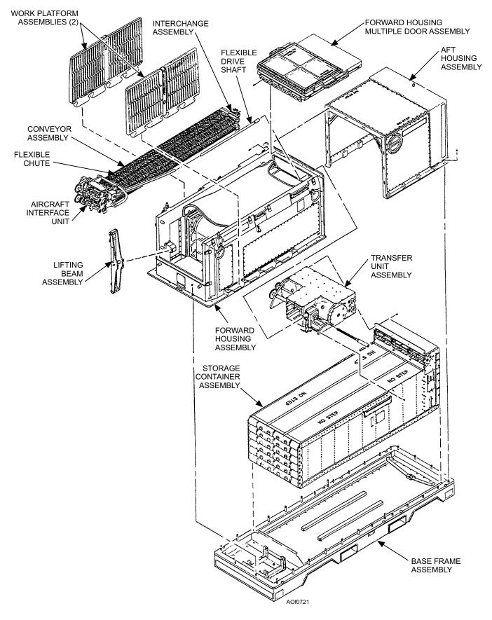
Figure 7-21.—Ammunition Loader.
