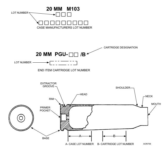
Figure 7-6.—M103 brass cartridge case and markings.
