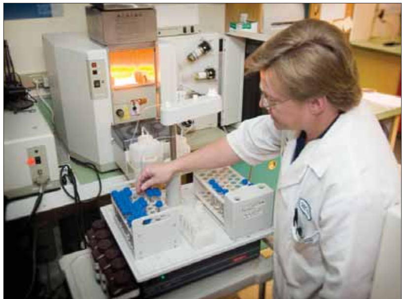
Above: Coachella Valley Water District chemist Mike Stenzel, a 14-year employee, tests water using an Atomic Absorption Spectrometer in the water district's state-certified laboratory.
