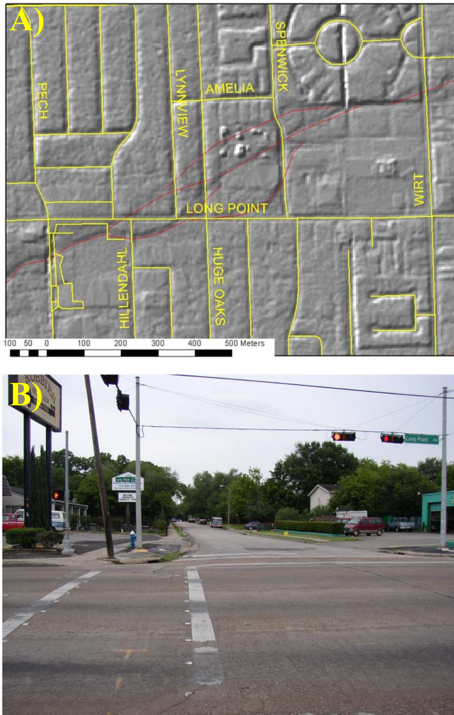
Figure 6. A) LIDAR hill-shade image of Long Point Fault where it crosses Long Point. Here the scarp bifurcates into several branches. B) Two separate scarps can be seen in the distance (highlighted by the red dashed lines). A third scarp has been interpreted further north but is subtle and gentle.
