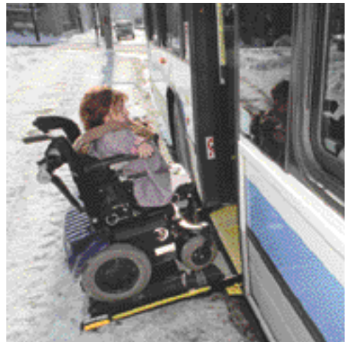
A retractable ramp has made the low-floor bus (LFS) accessible to persons in wheelchairs. (Michel E. Tremblay - STM)
