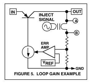
It is important to note that the signal starting at the  $V_B$  point has a phase shift introduced into it as it travels through the loop (eventually arriving at the  $V_A$  point). The amount of phase shift is critical in determining stability.
