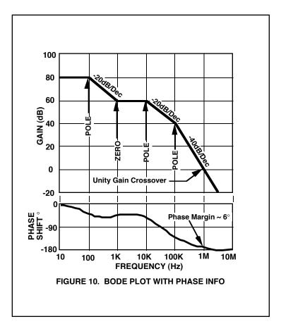
The plot of Phase Shift shows how the various poles and zeroes contribute their effect on the feedback signal. To produce this plot, the phase shift at each frequency point was calculated based upon summing the contributions of every pole and zero at that frequency. The phase shift at any frequency "f" which is caused by a pole located at frequency "f<sub>D</sub>" can be calculated from:
