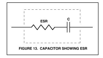
The frequency where the zero occurs is directly related to the value of the ESR and amount of output capacitance:
