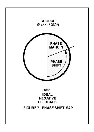
It can be seen that starting at -180°, an additional phase shift of 180° (positive or negative) brings the signal back to zero, which is the phase of the source signal and would cause the loop to be unstable.
