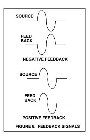
Positive feedback occurs when the feedback signal has the same polarity as the source signal. In this case, the loop responds in the same direction as any change which occurs at the output. This is clearly unstable, since it does not cancel out changes in output voltage, but amplifies them.
