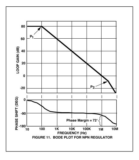
This dominant pole (shown as P1) for a typical NPN regulator is set at about 100 Hz. The 100 Hz pole causes the gain to decrease at a rate of -20 dB/decade until the second pole (P2) which is located at 3 MHz. At that point, the slope of the gain plot changes to -40 dB/decade.
